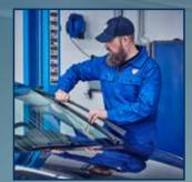
Remove the trim, seals and wipers in accordance with the vehicle manufacturer's instructions. Cut out the damaged windscreen using a cutting wire or a special knife. Use vacuum lifters to remove the defective windscreen.
