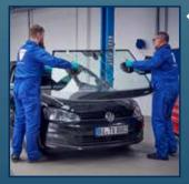
Insert the new windscreen within the adhesive's open time and use the tape to position it.
