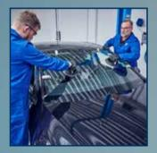
2 Before cleaning the new windscreen, we recommend testing its fit and inspecting it for defects. Now insert the spacers, if necessary, and use tape to mark the correct positions of the windscreen.
