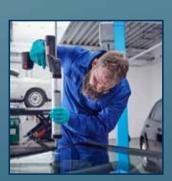
Apply windscreen adhesive as a triangular shaped bead either to the windscreen, the body flange, or the newly trimmed remaining bead.
