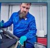
It is important to thoroughly clean the body flange with **DINITROL 582**, for example, before the remaining bead on the body flange is trimmed. Do not apply **DINITROL 582** or windscreen cleaning agent to the newly trimmed remaining bead. Let the flange briefly air dry after cleaning it.
